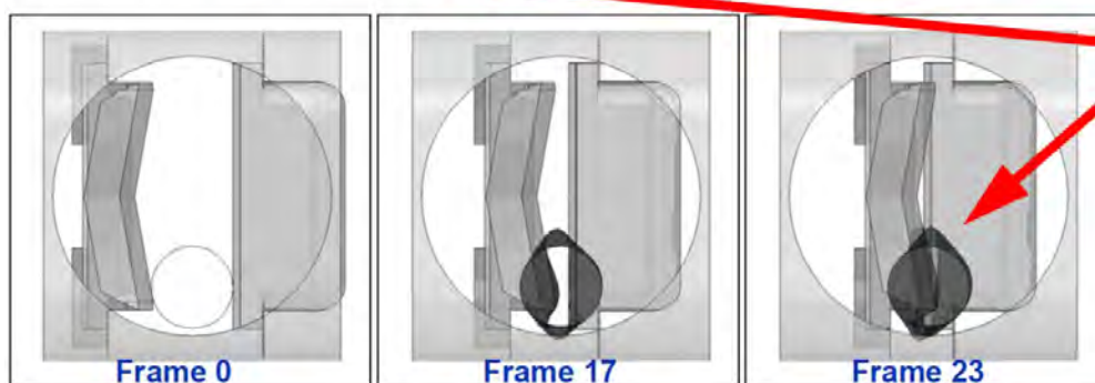
FIGURE 3-6 Progression of off-center BSR shear model, isometric view ( top ) and top view showing deformation of drill pipe outside of shearing blade surfaces ( bottom ). Source: DNV 2011b, p. 17. Reprinted with permission; copyright 2011, DNV.
